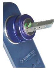
LC Transceiver Inspection
