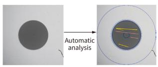
AutoCheck is the first intelligent integrated fiber end-face inspector developed by Dimension Technology. With the advantages of Dimension image analysis software and high performance embedded system, AutoCheck can identify the tiny defects accurately, conveniently and simply. The fiber end-face inspection complies with IEC standard and customized criteria.
